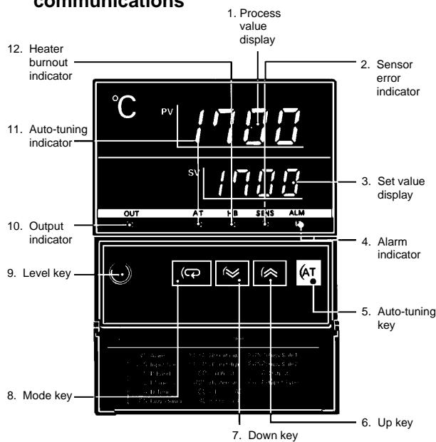
**E5AF-H Heater burnout controllers with communications**
