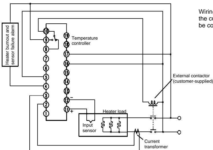
Wiring for the heaters must pass through the hole of the current transformer. The current transformer can be connected to the controller in any polarity.
